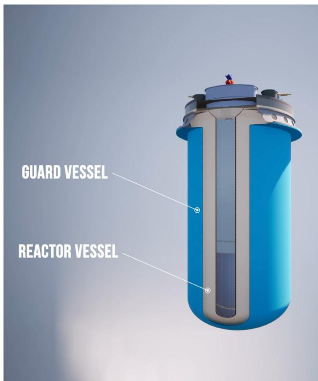
Figure 3-5 ARC-100 3-D Model Reactor Vessel
