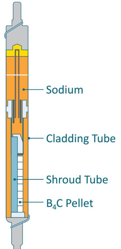
Figure 6-1 Shut-off Rod Schematic
