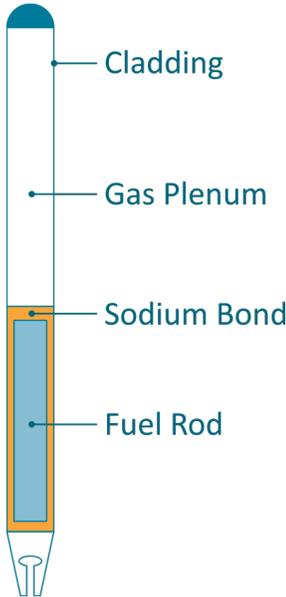
Figure 3-3 Schematic of a metal fuel pin, representative of ARC-100 Fuel
