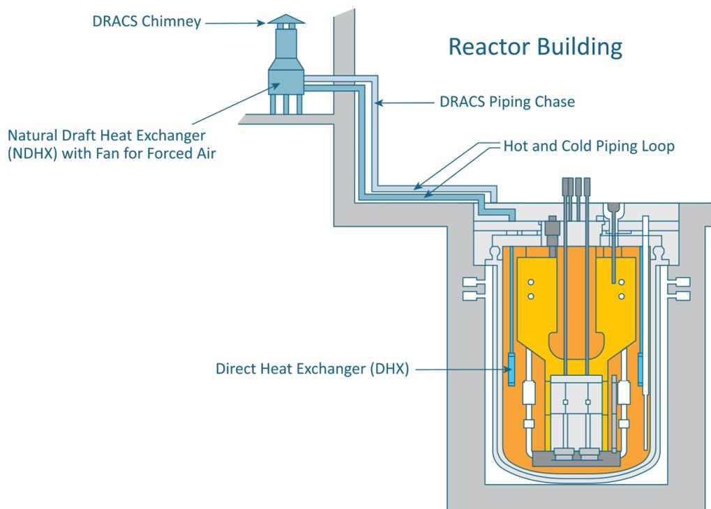
Figure 3-10 Direct Reactor Auxiliary Cooling System (DRACS) schematic
