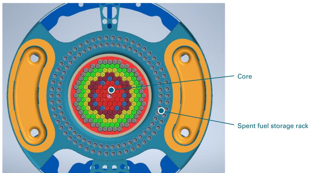
Figure 3-13 Top View of Fuel Storage Schematic
