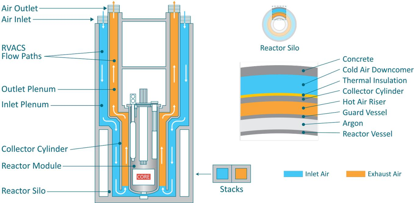
Figure 3-11 Reactor Vessel Auxiliary Cooling System (RVACS) schematic
